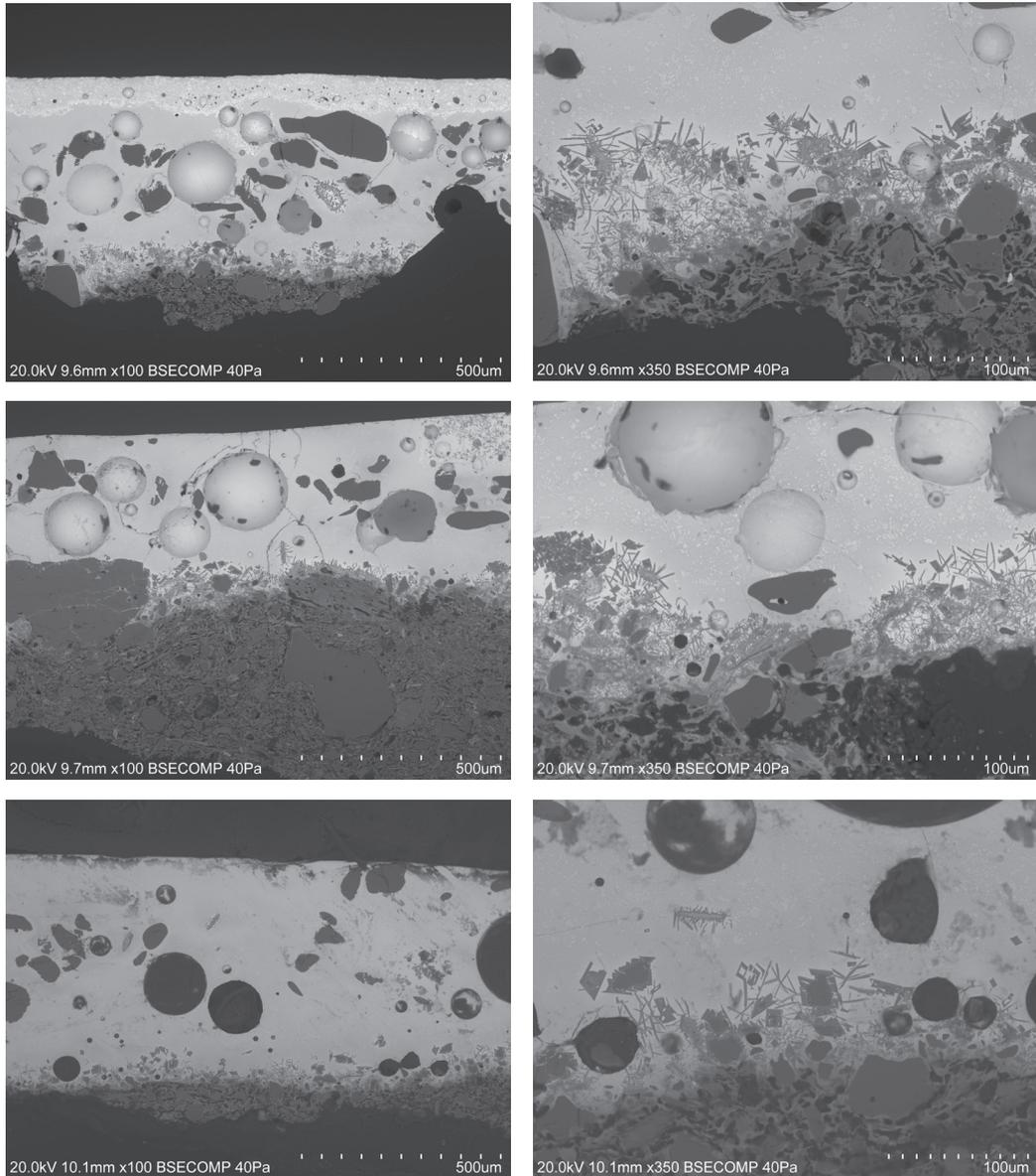
**Figure 7.** SEM images showing the glaze and the interfacial micro-morphology of azulejos from São Roque chapel – from top to bottom: samples Az068/02; Az068/03; and Az068/13 from tiles of the signed panel
