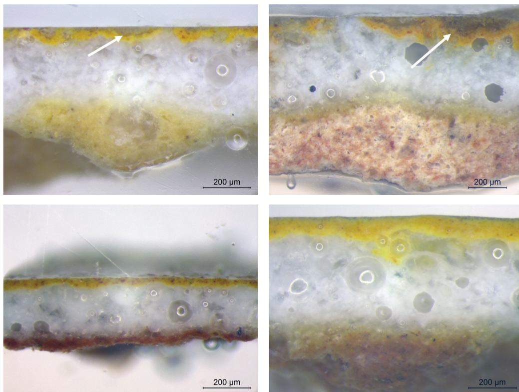
**Figure 4.** Top to bottom: use of sprinkled *coperta* in samples Az013/01 (left side) and Az013/L3 (right side) – the arrows indicate spots where drops of transparent glaze fell; absence of *coperta* in samples Az032/03 (left side) and Az068/02 (right side)
